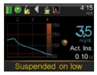
After the "Suspend on low" alert message is cleared, the screen will display: "Suspended on low" at the bottom of the screen in yellow print.
